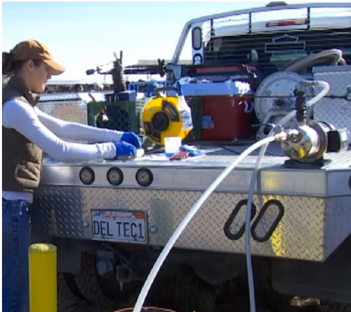
A CVDRMP well is sampled to measure depth to first-encountered groundwater, total dissolved solids, nitrogen and general minerals.
